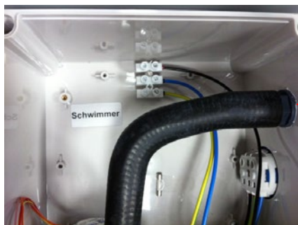
Figure 3: The hose inside the controller must not be twisted.
