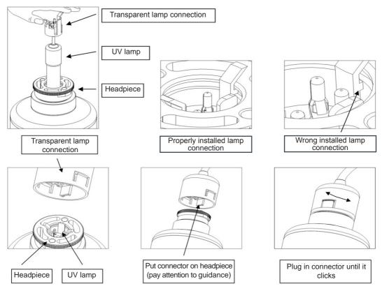
The quartz glass tube has to be cleaned at every maintenance, so 3 times per year, in order to ensure optimal operation (maximum cleaning interval four months!).
