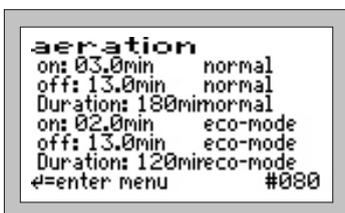
This menu is used to set for how many minutes the aerator should be turned ON or OFF (cycle).
