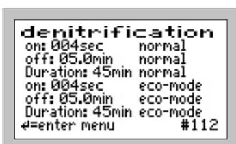
This menu is used to set for how many minutes the aerator should be turned ON or OFF. This is done for both normal operation and ecomode, but only for denitrification.
