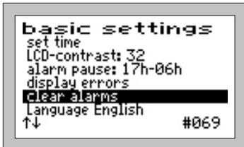
If a malfunction occurs (alarm), this can be reset by pressing the
