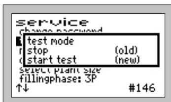
The automatic test mode is selected via the selection menu "start test".
