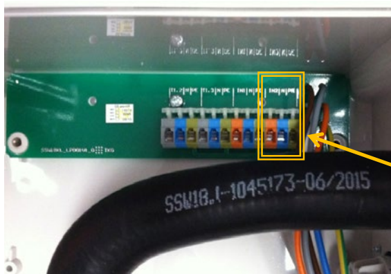
Figure 16: Connection of 2nd float switch as flood detector with K-Pilot 18.3
