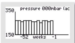
In the graphic menu "PRESSURE", the current pressure is documented in the upper line and the counterpressure (from the pressure monitoring) is documented on a weekly basis in the graphic.
