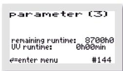
The Parameters 3 menu displays the "REMAINING RUNNING TIME" of the UV lamp and the total running time of the UV lamp as "UV OP. HRS". The settings of "REMAINING RUNNING TIME" are reset here to 2000 hours after the lamp has been changed.
