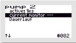
There are 3 options for "CURRENT MONITORING". The default presetting is "CONT." (= continuous), but it can also be set to "CYCLIC" or switched off entirely (display: "---"). If the "CYCLICAL" option was selected, the time period can be set in the "PARAMETERS (2)" menu (see Chapter 13.3.4.3).
