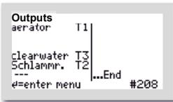
In this example, the compressor is controlled via output T1, the clear water discharge via output T3 and the sludge discharge via output T2.
