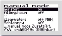
If a float switch is moved up and down, the indicator in the display changes accordingly.
