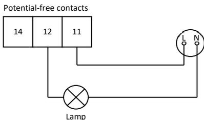
Figure 9: Potential-free contact with error indication – power supplied by controller
