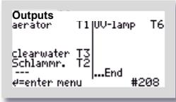
In this example, the compressor is controlled via output T1, clear water discharge via output T3, the sludge discharge via output T2 and the UV lamp via output T6. In addition, a UV lamp is controlled via output T6.
