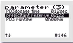
In the example, a dosing agent supply is set with a total dosing pump running time of 2 hours and 22 minutes.
