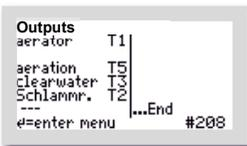
In addition, aeration is controlled via output T5 in this example.
