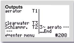
In this example, the three-phase compressor is selected as an additional function. A free output must be assigned to this function.
