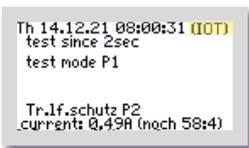
The test is fully automatic. The individual functions are tested in sequence (approx. 15 seconds each). If all the units are functioning correctly, no alarm message is issued.
