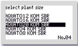
For plant sizes from 21 to 50 PE, please select "AQUATO>20 KQM SBR". The cycle presets for plant sizes from 21 to 50 PE are the same; the different air volumes required are reached with different sizes and volumes of membrane diffusers and compressors. These settings can be readjusted where necessary.
