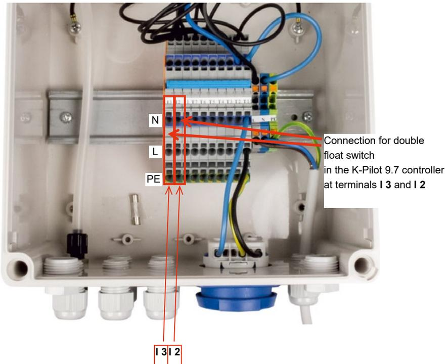
Figure 14: Connection of double float switch to K-Pilot 9.7 controller
