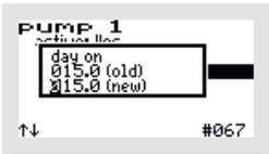
The running times of the pumps are set here. The "ON" switching time and the "OFF" switching time can be set independently of each other. They then take place in alternation.
