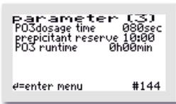
The Parameters 3 menu displays the "PO3 DOSING TIME" per cycle, the "DOSING AGENT SUPPLY" and the total running time of the dosing pump as "PO3 OP. HRS". The settings "PO3 DOSING TIME" per cycle and "DOSING AGENT SUPPLY" can also be adjusted here.
