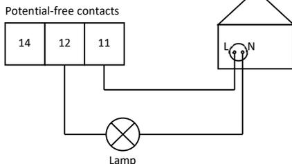
Figure 10: Potential-free contact with error indication even in case of power failure
