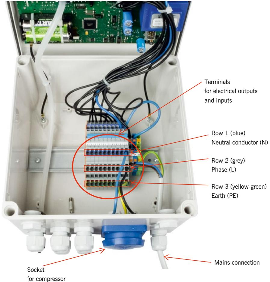
Figure 5: Electrical connections of the K-Pilot 9.7 controller
