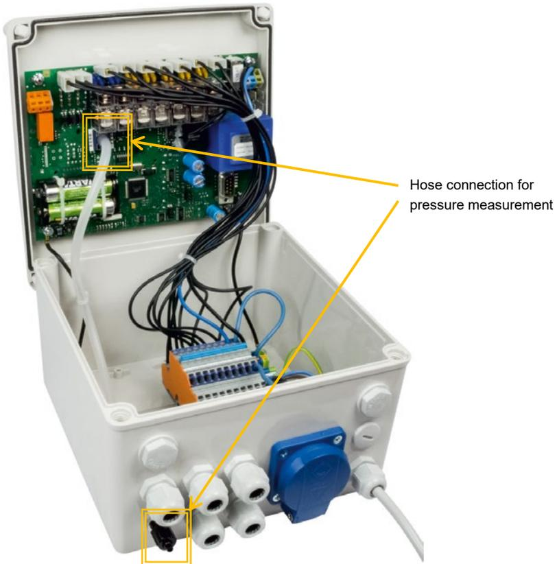
Figure 3: Connection for pressure measurement on and in the controller
