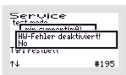
In the next window, "HW error deactivated" the flooding error message can be deactivated. This is usually unnecessary. After confirming the selection, the next window opens automatically.
