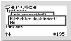
In the next window, "HW error deactivated" the flooding error message can be deactivated. This is usually unnecessary. After confirming the selection, the next window opens automatically.
