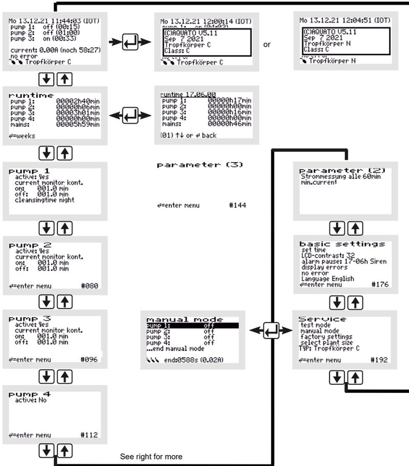
Figure 23: Menu structure of Trickling Filter C and Trickling Filter N
