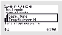
For operation as a trickling filter plant with 3 pumps and 2 floats, please select "**TRICKLING FILTER C**". For operation as a trickling filter plant with 2 pumps and 2 floats, please also select "**TRICKLING FILTER C**". For operation as a trickling filter plant with 2 pumps and 1 float, please select "**TRICKLING FILTER N**".
