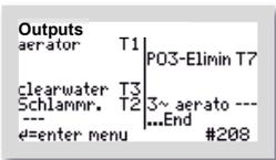
If one or more additional functions – in this example PO3 elimination and the three-phase compressor – have been selected, a separate output must be assigned to each of these functions. This can be seen from the blank space symbols "—" after the units.
