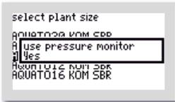
If you switch on the monitoring by selecting "YES" in the menu "WITH PRESSURE MONITORING", an error message will be generated if the device fails. **To use this monitoring, the pressure sensor must be connected to the air hose between the compressor and the diffusers.** If the sensor is not connected to the air hose, select "NO".
