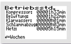
The operating hours of the individual units are displayed in the OPERATING HOURS chapter for your controller. The operating hours are counted up if the controller has switched on the compressor (or possibly the pump if the K-Pilot 18.3 controller is in use). The display is in hours and minutes.
