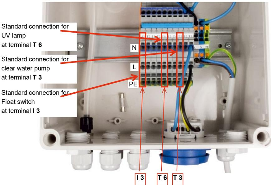
Figure 25: K-Pilot 9.7 controller – UV lamp connection
