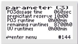
In the example, a dosing pump for phosphate precipitation and a UV module are connected. In this case, the data regarding the dosing agent supply and the dosing time can be adjusted and the remaining UV time can be reset.
