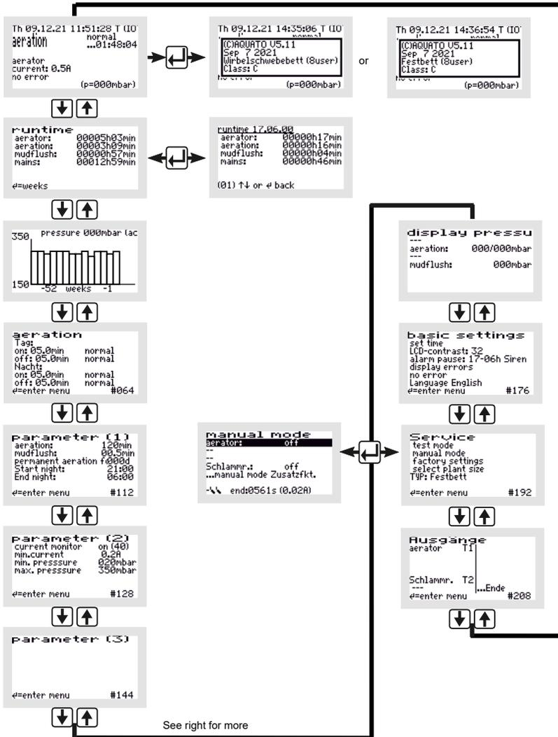
Figure 21: Menu structure for fluidised/fixed bed plant
