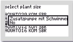
If the additional pump is to be operated with an external float switch, please use the buttons to select the option "YES" in the "ADDITIONAL PUMP WITH FLOAT" window.
