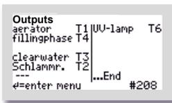
If, as in the example, the "UV Lamp" function was assigned to output T 6, the electrical connection for the hygienisation (here: with a UV lamp) must also be connected to contact T 6. In the example, the "CLEAR WATER PUMP" function was also assigned to output "T1.3", so the electrical connection of the clear water pump must also be connected to contact T1.3.
