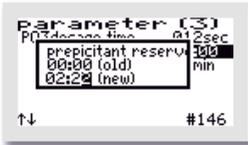
The stored quantity of the dosing agent is not entered directly, but rather the total dosing pump running time for which the supply is adequate. (Calculation in operating manual for P precipitation)
