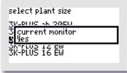
If you switch on the monitoring by selecting "YES" in the menu "CURRENT MONITORING", an error message will be generated if the device fails.
