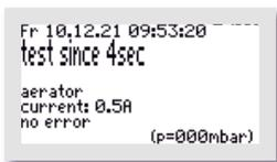
The test is fully automatic. The individual functions are tested in sequence (approx. 15 seconds each). If everything is functioning correctly, no alarm message is issued.
