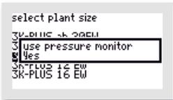
If you switch on the monitoring by selecting "YES" in the menu "WITH PRESSURE MONITORING", an error message will be generated if the device fails.
