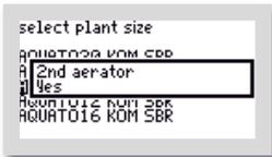
If you are operating a plant with 2 (or 3) compressors, please use the buttons to select "YES" in the window with the query "2nd COMPRESSOR".
