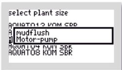
If the surplus sludge discharge is equipped with a submersible motor pump instead of the compressed air lifter, please select "MOTOR PUMP" in the "SLUDGE DISCHARGE" window.
