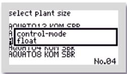
To operate a system with UV lamp or a dosing unit, the "FLOAT" control type must be selected.
