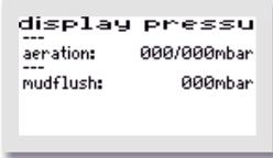
This menu displays the respective pressure during the last cycle. The aeration and surplus sludge counterpressures are each stored for each individual process. Only the pressure measurement of the respective last phase is displayed.
