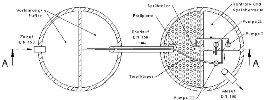
Figure 22: Trickling filter plant with pumps
