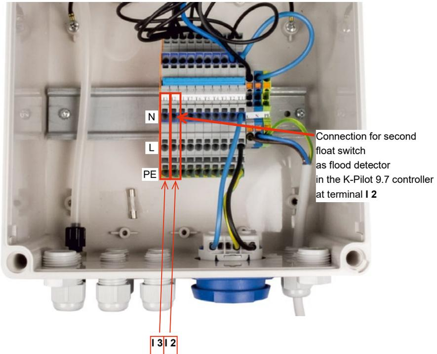
Figure 13: Connection of 2nd float switch as flood detector
