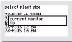
If you have selected "YES" for the query "3~COMPRESSOR", you will be asked in the "CURRENT MONITORING" window whether the three-phase compressor should be monitored for current errors. If you do not require this monitoring, you can switch it off with "NO".
