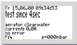
The test runs fully automatically as a standard test. It is independent of the selected program. The individual functions are tested in sequence (approx. 15 seconds each). If everything is functioning correctly, no alarm message is issued.
