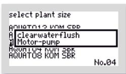
If the clear water discharge is equipped with a submersible motor pump instead of the compressed air lifter, please select "MOTOR PUMP" in the "CLEAR WATER DISCHARGE" window.
