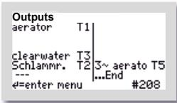
In this example, the compressor is controlled via output T1, the clear water discharge via output T3 and the sludge discharge via output T2. In addition, a three-phase compressor is controlled via output T5.
