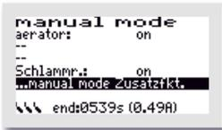
Three float switch symbols indicating the current float position are visible at the bottom left of the display.
