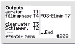
If, as in the example, the "UV Lamp" function was assigned to output T 7, the electrical connection for the hygienisation (here: with a UV lamp) must also be connected to contact T 7.
