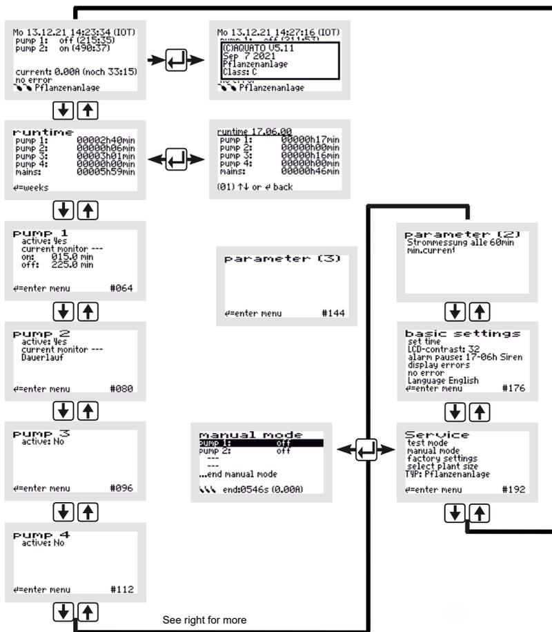
Figure 24: Menu structure of Tricking Filter C and Tricking Filter N
