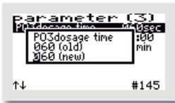
In the example, the PO3 dosing time is being changed from 60 to 12 seconds per cycle.
