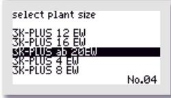
For plant sizes from 21 to 50 PE, please select "3K-FLOW from 20" or "3K-PLUS from 20". The cycle presets for plant sizes from 21 to 50 PE are the same; the different air volumes required are reached with different sizes and volumes of membrane diffusers and compressors. These settings can be readjusted where necessary.
