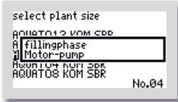
If the charging is equipped with a submersible motor pump instead of the compressed air lifter, please select "MOTOR PUMP" in the "CHARGING" window.
