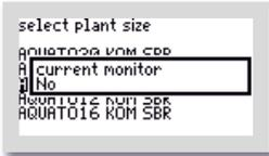
If you have selected a three-phase compressor, you will be asked in the "CURRENT MONITORING" window whether the three-phase compressor should be monitored for current errors. If you do not require this monitoring, you can switch it off with "NO".
