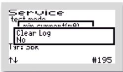
The last window to open in this menu is "DELETE LOG". If "YES" is selected here, all entries and settings are deleted. Then the controller starts over again with commissioning.
