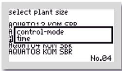
The "CONTROL TYPE" window allows you to choose between a time-controlled cycle or a float-controlled cycle. The desired control type can be set in the second line. Press the buttons to select "TIME" or "FLOAT". The selected Control type is accepted with the button. If "TIME" is selected, the cycle sequence is only controlled through time, but if "FLOAT" is selected, it is also float-controlled.
