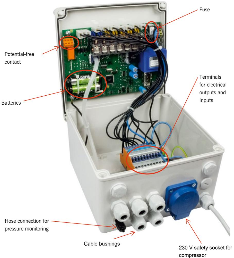
Figure 2: K-Pilot 9.7 controller opened
