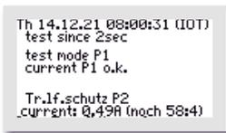
The test is fully automatic. The individual functions are tested in sequence (approx. 15 seconds each). If all the units are functioning correctly, no alarm message is issued.
