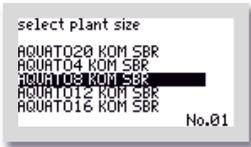
Then use the buttons to select the desired/required EW number as the "PLANT TYPE". If the marker (= black bar) is on the correct PE number (according to the wastewater treatment calculation), confirm with the button. If the required PE number is not directly available for selection, select the next largest entry.
