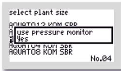
If you switch on the monitoring by selecting "YES" in the menu "WITH PRESSURE MONITORING", an error message will be generated if the device fails. **To use this monitoring, the pressure sensor must be connected to the air hose between the compressor and the diffusers.** If the sensor (hose connection for pressure monitoring, see Figure 4) is not connected to the air hose, select "NO".
